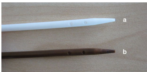
Fig. 3 Visual comparison of a untreated catheter b silver-treated catheter
